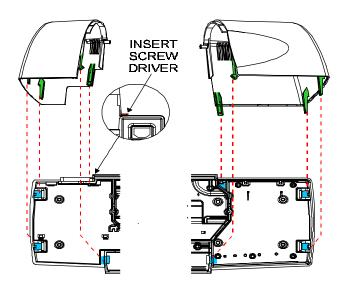
Figure 5-1. Cover Removal/Installation.
